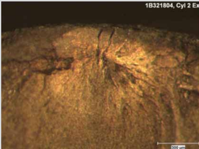
Figure 1: Stereo microscope image showing a classic fatigue halo.
